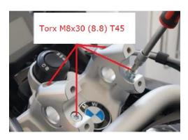
The original clamp parts are fitted with original screws (please proceed according to the manufacturing book!). The upper clamp must be mounted without any gap. See pictures below. Check the screws regularly for a tight fit! Torque: 23Nm
